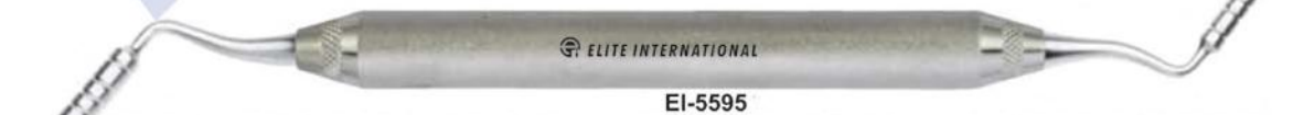
EI-5595 Titanium graft packer/ placement site depth gauge 3.3mm & 4.0mm Diameter tips Marked at 8, 11, 13, 15 & 18mm
